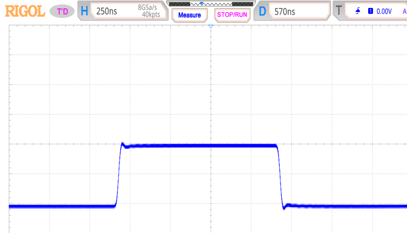
Fig. 3. Single-polar rectangular excitation pulse of a flux-gate transmitter
